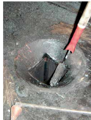
Continuous casting mould for billets: coating with fibre roller
