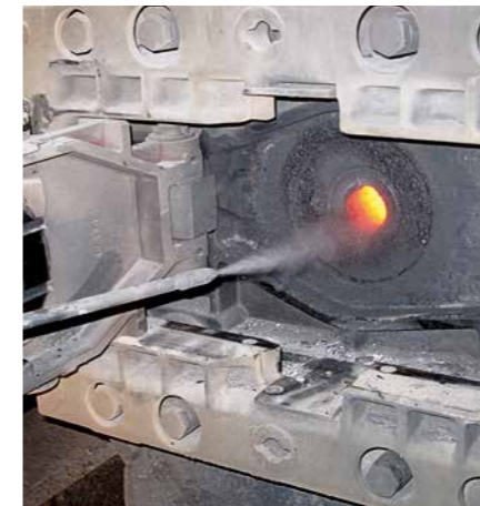
Hot-spraying, sealing surface ladle nozzle / sliding bottom plate
