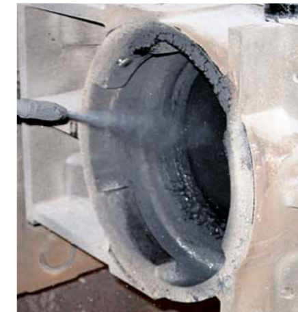
Hot-spraying, sealing surface sliding plate / exchangeable nozzle
