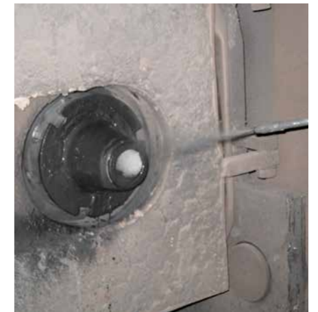
Hot-spraying, sealing surface exchangeable nozzle / ladle-shroud
