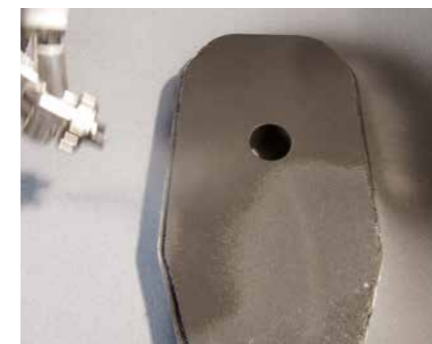
Surface coating (spraying) of linear sliding plate
