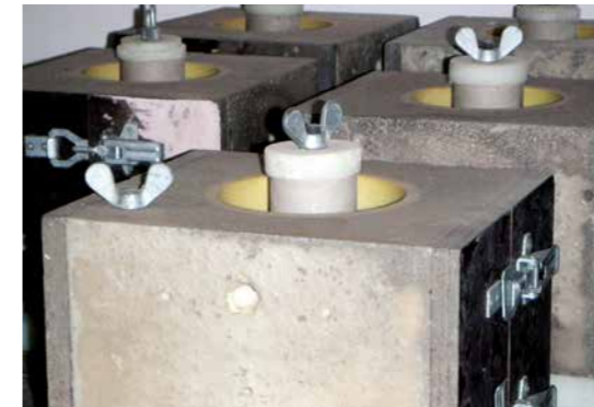
Casting mould for the production of cast ceramic components
