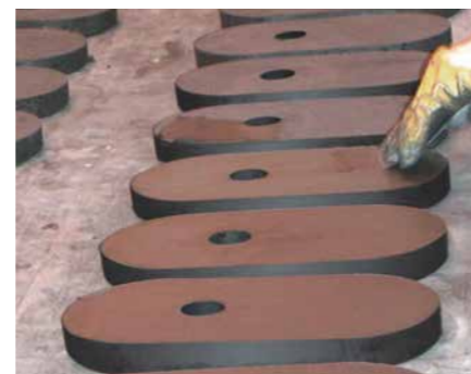
Manual surface coating of ceramic sliding plates
