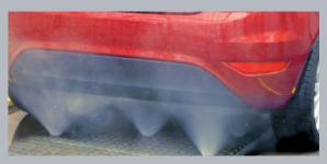
Possible choice: static underchassis wash 10 bar [145 PSI] 90 L/min [23.8 gpm], oscilating 15 bar [217 PSI] 120 L/min [31.7 gpm], or by sector 15 bar [217 PSI] 120 L/min [31.7 gpm].
